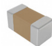
C0603C103J3RACTU KEMET CAP CER 10000PF 25V X7R 0603
