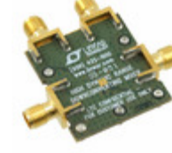
DC1885A Linear Technology EVAL BOARD DOWNCONVERTER LTC5544
