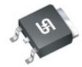
TSM70NB1R4CP ROG TSC (Taiwan Semiconductor) MOSFET N-CHANNEL 700V 3A TO252
