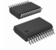
ICL3217IAZ-T Intersil IC 5DRVR/3RCVR RS232 3V 24-SSOP
