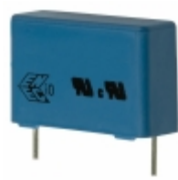
B81122A1473M EPCOS (TDK) CAP FILM 0.047UF 20% 250VAC RAD
