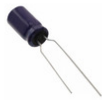
ECA-2DM3R3 Panasonic Electronic Components CAP ALUM 3.3UF 20% 200V RADIAL
