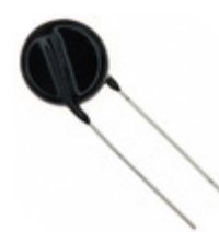
ERZ-V20D270 Panasonic Electronic Components VARISTOR 27V 3KA DISC 20MM
