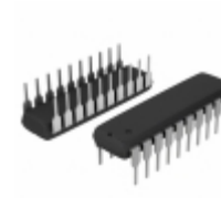
PIC16C770-E/P Microchip Technology IC MCU 8BIT 3.5KB OTP 20DIP
