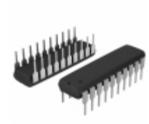
PIC16C770-I/P Microchip Technology IC MCU 8BIT 3.5KB OTP 20DIP
