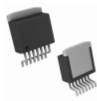
MIC49500-1.2WU TR Microchip Technology IC REG LDO 1.2V 5A TO263-7
