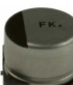
EEE-FK1V151P Panasonic Electronic Components CAP ALUM 150UF 20% 35V SMD
