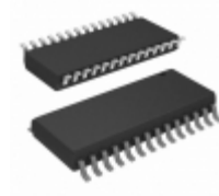
ICL3238ECA Intersil IC 5DRVR/3RCVR RS232 3V 28-SSOP
