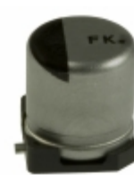
EEV-FK1H100UR Panasonic Electronic Components CAP ALUM 10UF 20% 50V SMD
