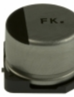
EEV-FK1H101GP Panasonic Electronic Components CAP ALUM 100UF 20% 50V SMD
