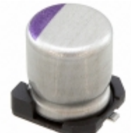
10SVPS15M Panasonic Electronic Components CAP ALUM POLY 15UF 20% 10V SMD
