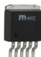
MIC37502BU TR Microchip Technology IC REG LDO ADJ TO263-5
