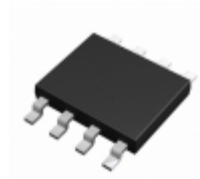
BU7242SFVM-TR Rohm Semiconductor IC OPAMP GP 900KHZ RRO 8MSOP
