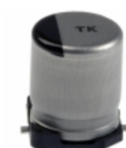
EEE-TK1C221UP Panasonic Electronic Components CAP ALUM 220UF 20% 16V SMD
