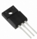
BA33DD0T Rohm Semiconductor IC REG LDO 3.3V 2A TO220FP
