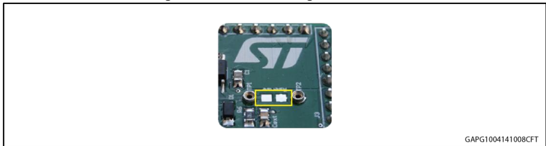
Figure 5: Pads for soldering SMD resistor
