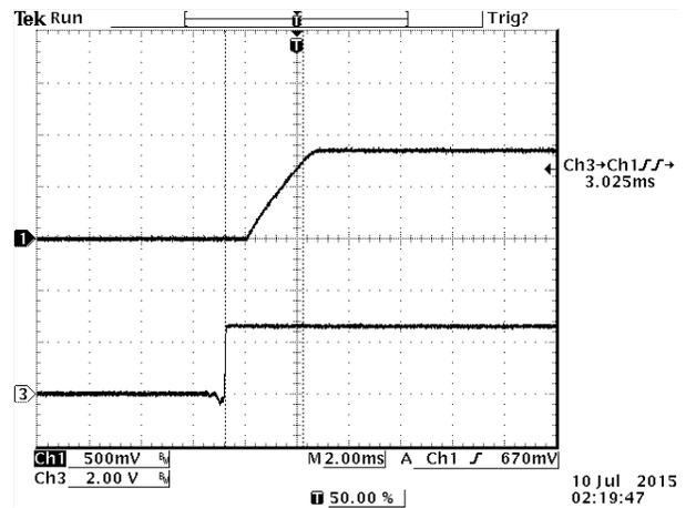
Figure 25. Startup time at full load, 12 VDC input
