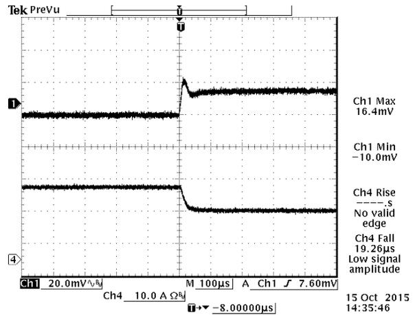
Figure 17.  $V_{in} = 75\% - 50\%$  Load Transient at  $V_{in} = 12\text{ VDC}$
