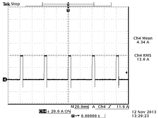
Figure 34. Output current @ SCP,  $V_{in} = 12\text{ V}$
