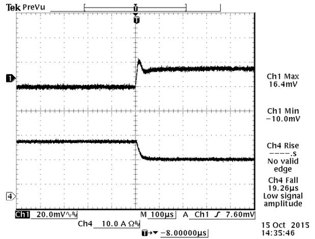
Figure 19.  $V_{in} = 75\% - 50\%$  Load Transient at  $V_{in} = 12\text{ VDC}$
