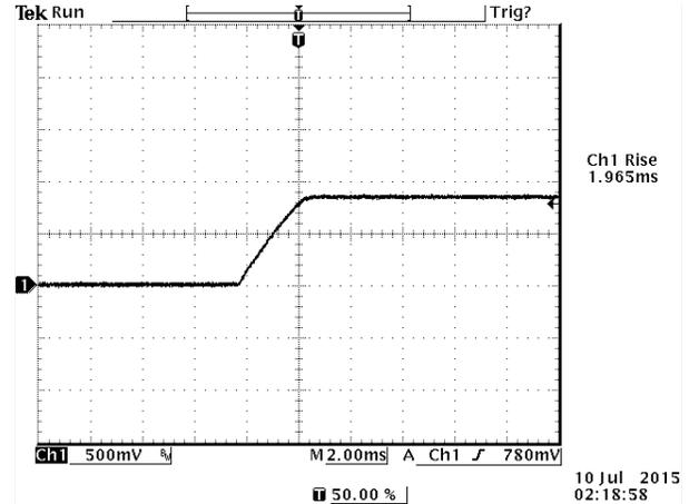
Figure 22. Rise time at full load, 12 VDC input
