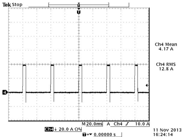
Figure 33. Output current @ SCP,  $V_{in} = 12\text{ V}$
