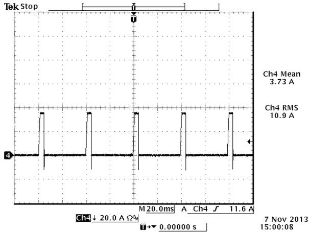
Figure 31. Output current @ SCP,  $V_{in} = 12\text{ V}$
