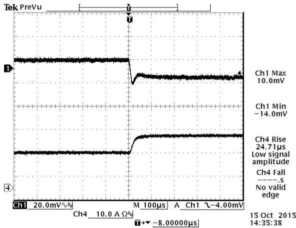
Figure 16.  $V_{in} = 50\% - 75\%$  Load Transient at  $V_{in} = 12\text{ VDC}$
