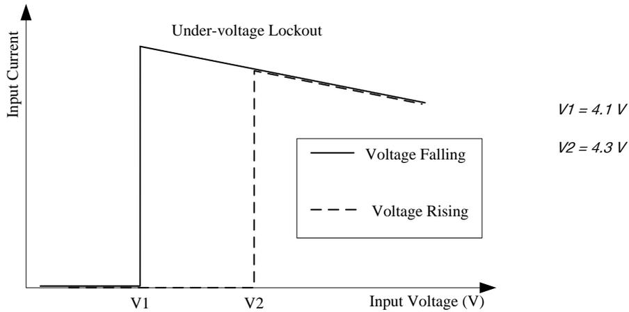
Figure 20. Input under-voltage lockout
