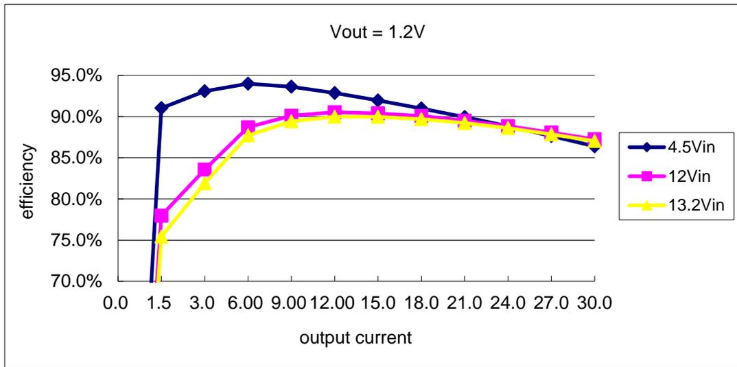
Figure 2. Efficiency @ Vo = 1.2 V
