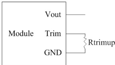
Figure 27. Trim up circuit (using an external resistor)
