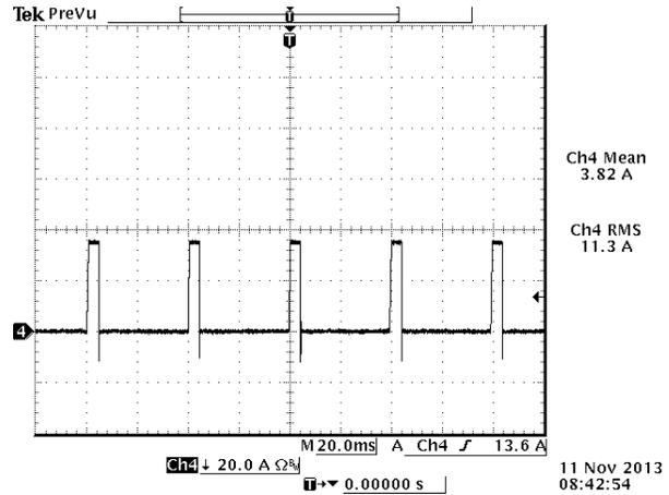
Figure 32. Output current @ SCP,  $V_{in} = 12\text{ V}$
