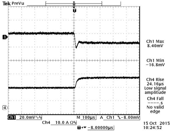
Figure 14.  $V_{in} = 50\% - 75\%$  Load Transient at  $V_{in} = 12\text{ VDC}$
