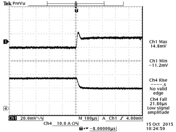
Figure 15.  $V_{in} = 75\% - 50\%$  Load Transient at  $V_{in} = 12\text{ VDC}$
