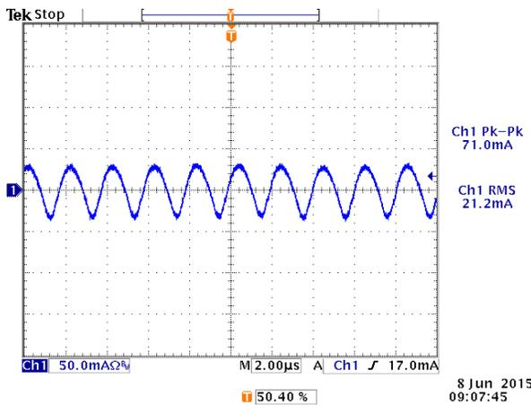
Figure 5. is (input terminal ripple current), AC component
