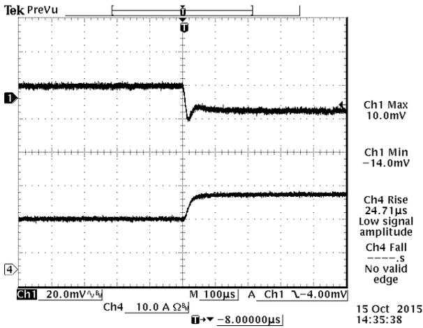
Figure 18.  $V_{in} = 50\% - 75\%$  Load Transient at  $V_{in} = 12\text{ VDC}$
