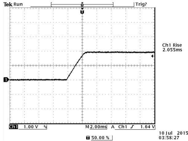
Figure 23. Rise time at full load, 12 VDC input
