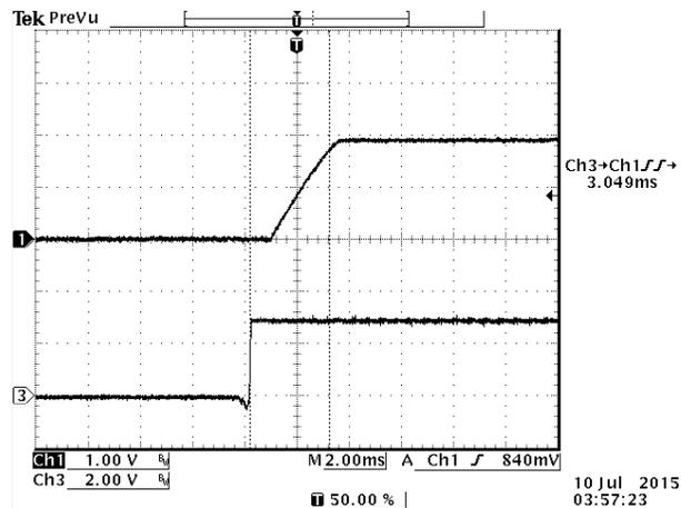
Figure 26. Startup time at full load, 12 VDC input
