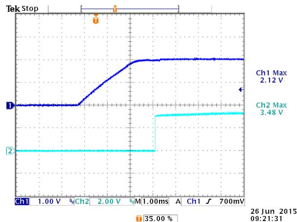
Figure 35. Typical Start-up using Remote on/off,
