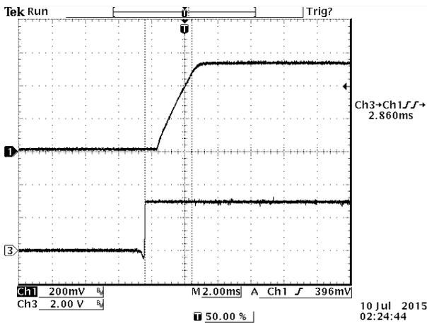
Figure 24. Startup time at full load, 12 VDC input
