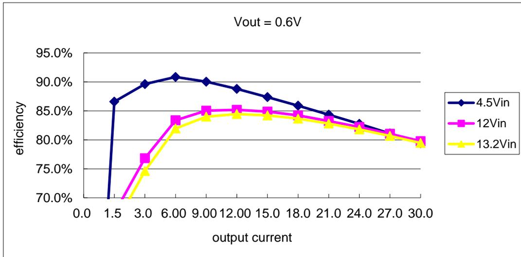
Figure 1. Efficiency @ Vo = 0.6 V
