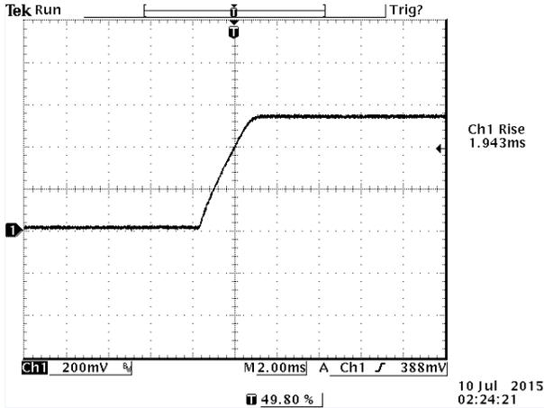
Figure 21. Rise time at full load, 12 VDC input
