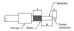
2) Position the contact on to the centre conductor and against the dielectric, crimp the contact using the toll indicated.
