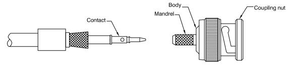
3) Insert the contact into the body and ensure that the contact captivates. Make sure that the braid is on the outside of the mandrel. Slide the ferrule over the braid until the ferrule butts up against the body. Crimp the ferrule using the tool indicated.
