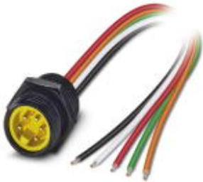
Flush-type connector, 5-position, Plug, straight, 7/8"-16UNF, on free cable end, Front mounting, with 1/2 inch-14 NPT mounting thread, Individual wires, cable length: 1 m
