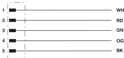
Contact assignment of the 7/8" plug
