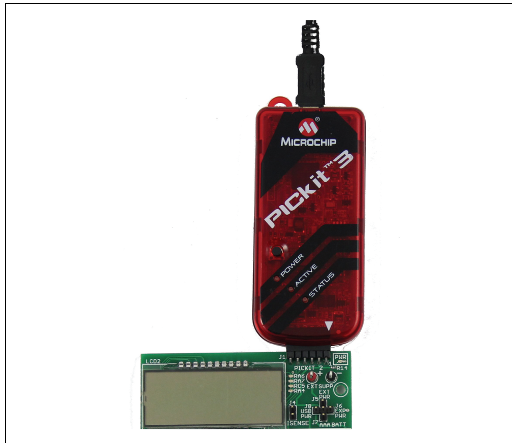
FIGURE 2-2: POWERING FROM PICKit™ 3
