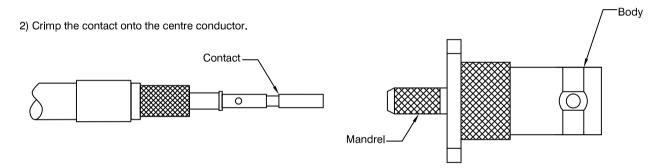
3) Insert the contact into the body and ensure that it captivates. Make sure that the braid is on the outside of the mandrel. Slide the ferrule over the braid until the ferrule butts up against the body. Crimp the ferrule using the correct tool for the connector.
