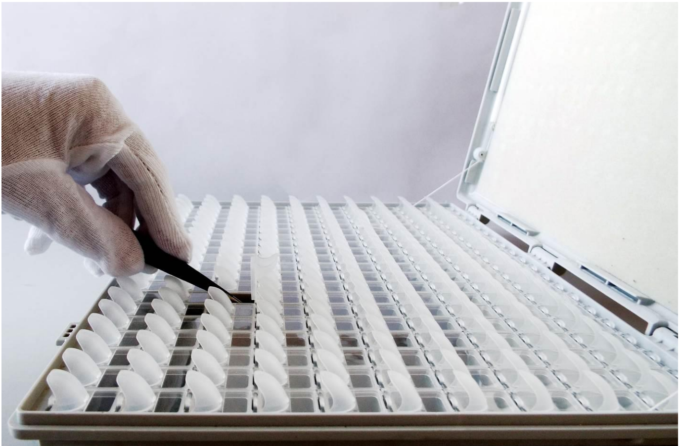
Figure 17. Store or Get an SMT Component with Single-Hand Operation
