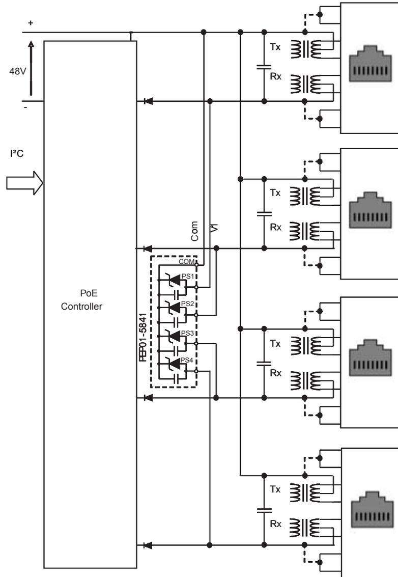
Figure 11. Typical application circuit with external PMOS
