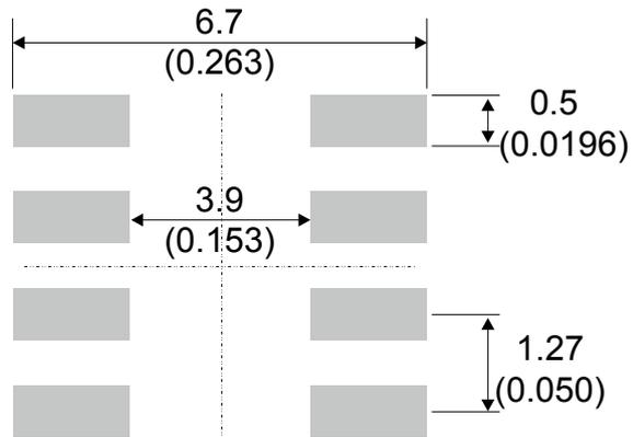
On top of the recommended SO-8 footprint described in Figure 14. Footprint recommendations, dimensions in mm (inches), the above footprint offers a better clearance for voltage higher than 50 V.
