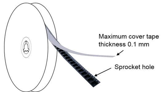
**Figure 18. Reel dimensions (mm)**
