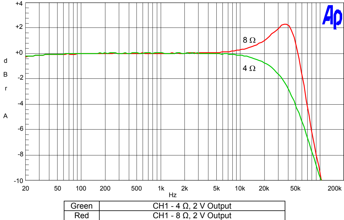
Figure 18. Frequency Characteristics vs. Load Impedance
