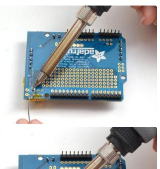
Then flip the board over and solder the 6 pins
