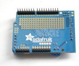
Finally, break off a 2-pin piece of header and place it next to the POWER terminal block, short legs down, tape it in place if necessary and solder it in.
