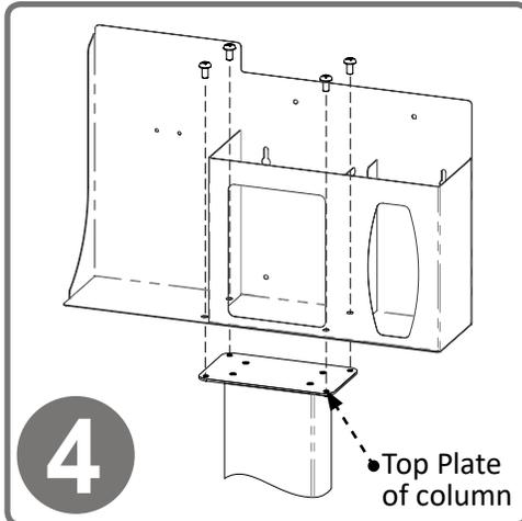
Attach the RS004-0212 Respiratory Hygiene Station to the column using (4x) screws included with stand. Tighten.
