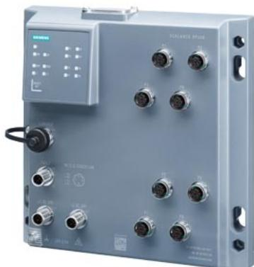
SCALANCE XP208 (EIP), managed IE switch, 8x 10/100 Mbit/s M12 ports, IP65, LED diagnostics, error signaling contact, redundant power supply, IEC 62443-4-2 certified; Ethernet/IP, network management, including dust caps, including electronic manual on CD-ROM, C-plug optional.
