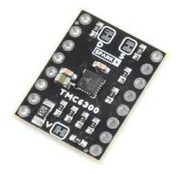
The TMC6300 from Trinamic is a powerful, yet easy to use three phase brushless DC (BLDC) motor driver. Separate high side and low side controls allow for incredible control up to 2A of current. The driver is temperature and short circuit protected with a diagnostic output pin to indicate system issues. With an operating voltage down to 2V, the TMC6300 is suitable for battery powered designs.
