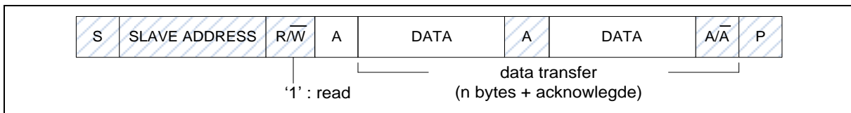
Figure 6.11-8 Master Reads Data from Slave by 7-bit
