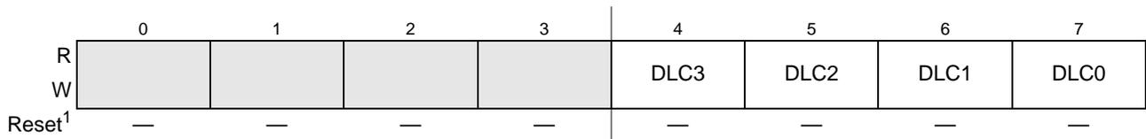
**Figure 22-29. Data Length Register (DLR)—Extended Identifier Mapping**
