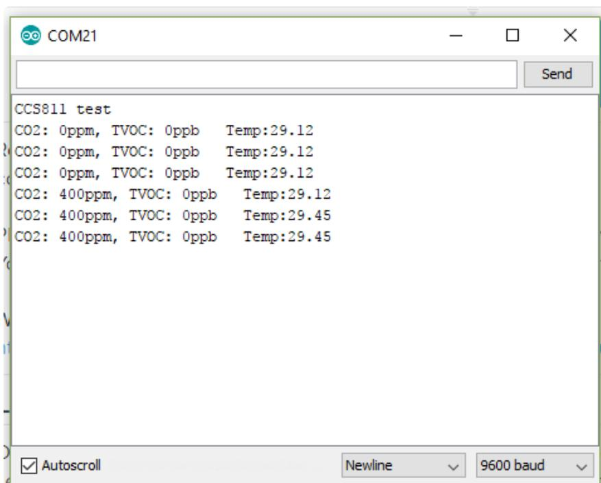
AMS recommends that you run this sensor for 48 hours when you first receive it to "burn it in", and then 20 minutes in the desired mode every time the sensor is in use. This is because the sensitivity levels of the sensor will change during early use.
