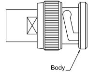
4) Insert the cable and parts into the connector body. Tighten the clamp nut using the appropriate wrenches.
