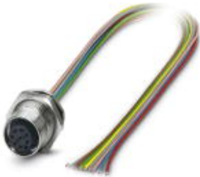
Sensor/actuator flush-type socket, 8-pos., M12 SPEEDCON, rear/screw mounting with Pg9 thread, with 0.5 m TPE litz wire, 8 x 0.25 mm 2
