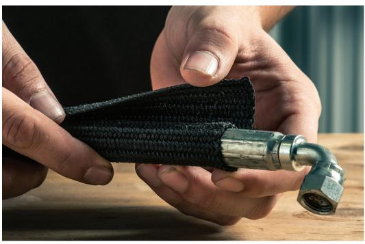
F6® HEAVY Wrap is specially designed to protect high voltage battery cables in hybrid and electric vehicles from crash and cut-through damage. It also allows to avoid short circuit on power lines by isolating the electrical system from the rest of the vehicle. F6H keeps wiring harness systems safe and secure in case of accidents; driver and passengers protection but also safety teams against high electrical loads.
