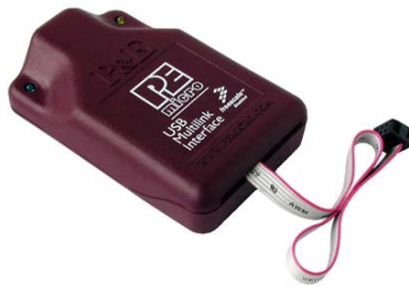
Figure 10-1: P&E's USB Multilink (USB-ML-12 shown)
