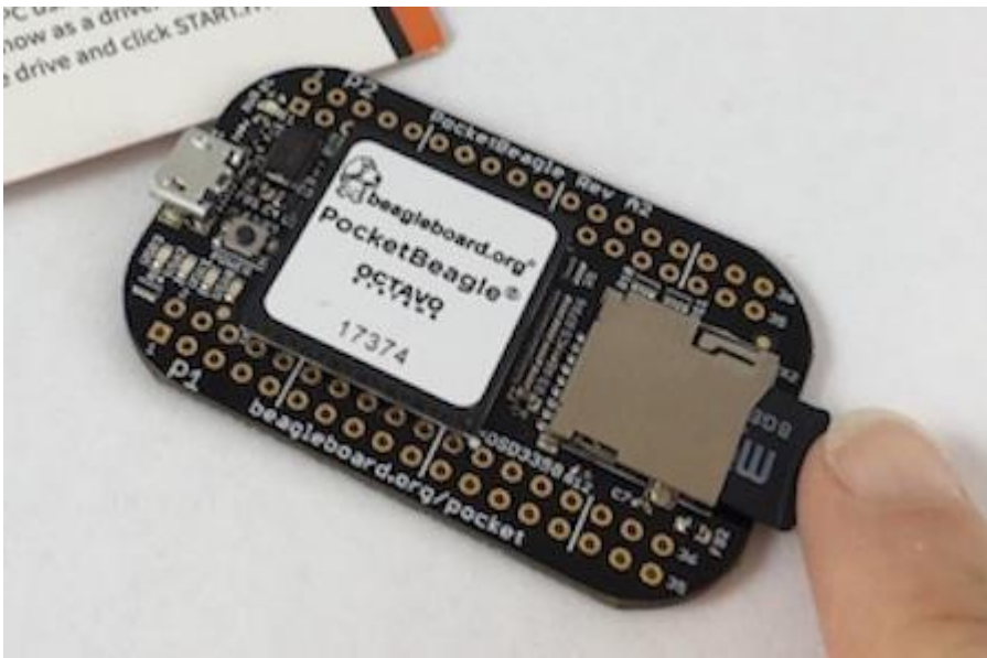
Figure 10. Insert the microSD Card into PocketBeagle
