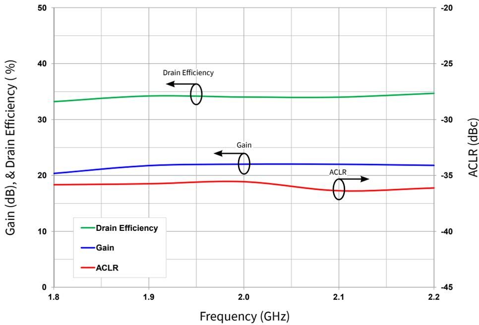
**Figure 9.** Typical Gain, Drain Efficiency and ACLR vs Frequency
