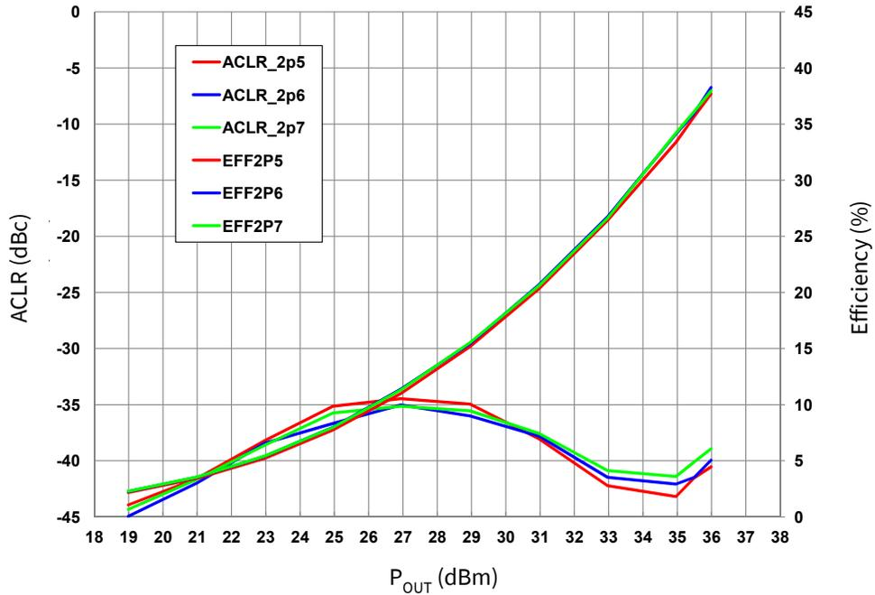
**Figure 5.** Typical Drain Efficiency and ACLR vs. Output Power
