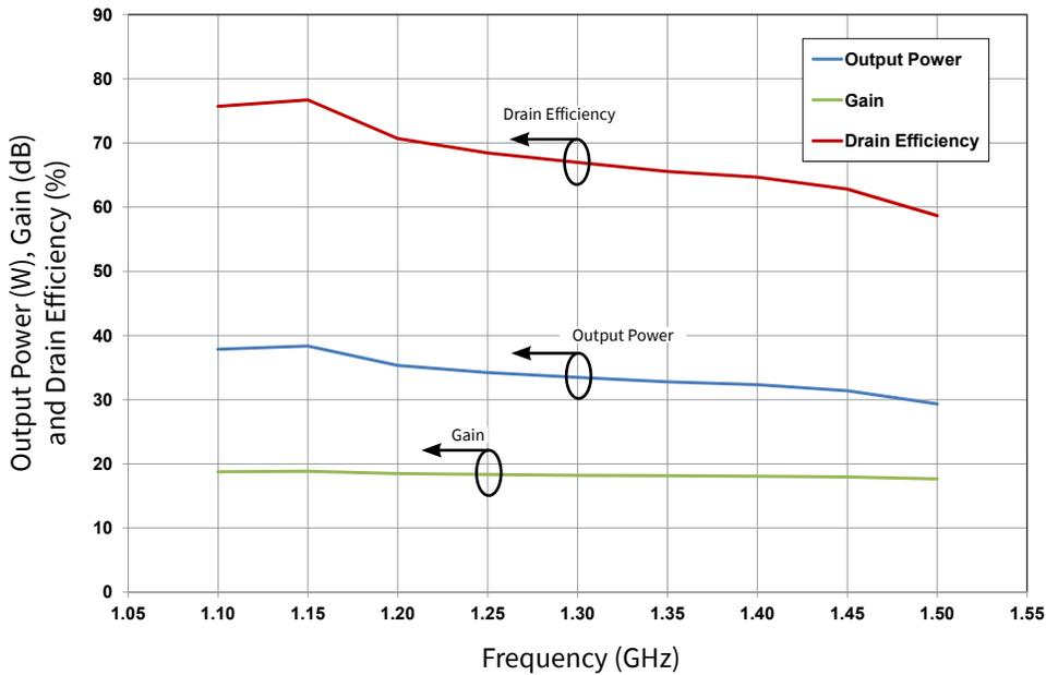
**Figure 15.** Typical Output Power, Gain, and Drain Efficiency vs Frequency
