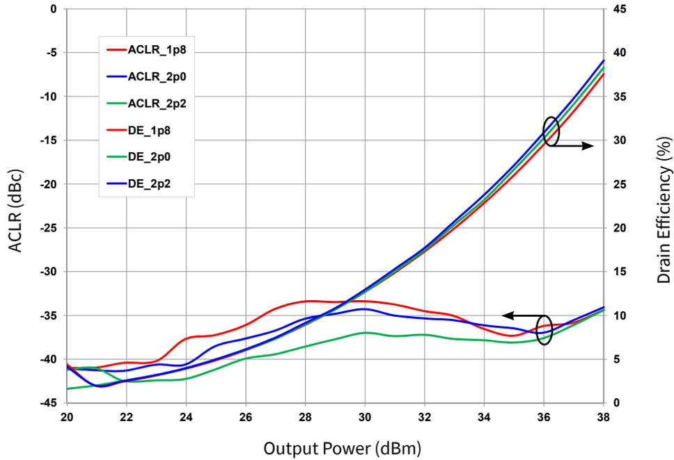
**Figure 11.** Typical Drain Efficiency and ACLR vs. Output Power
