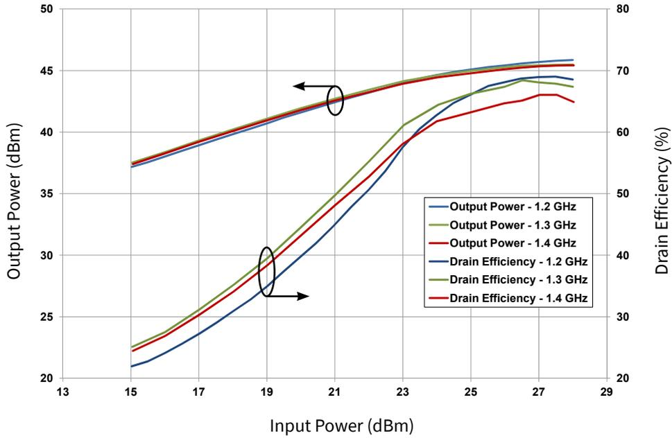
**Figure 14.** Typical Output Power and Drain Efficiency Input Power
