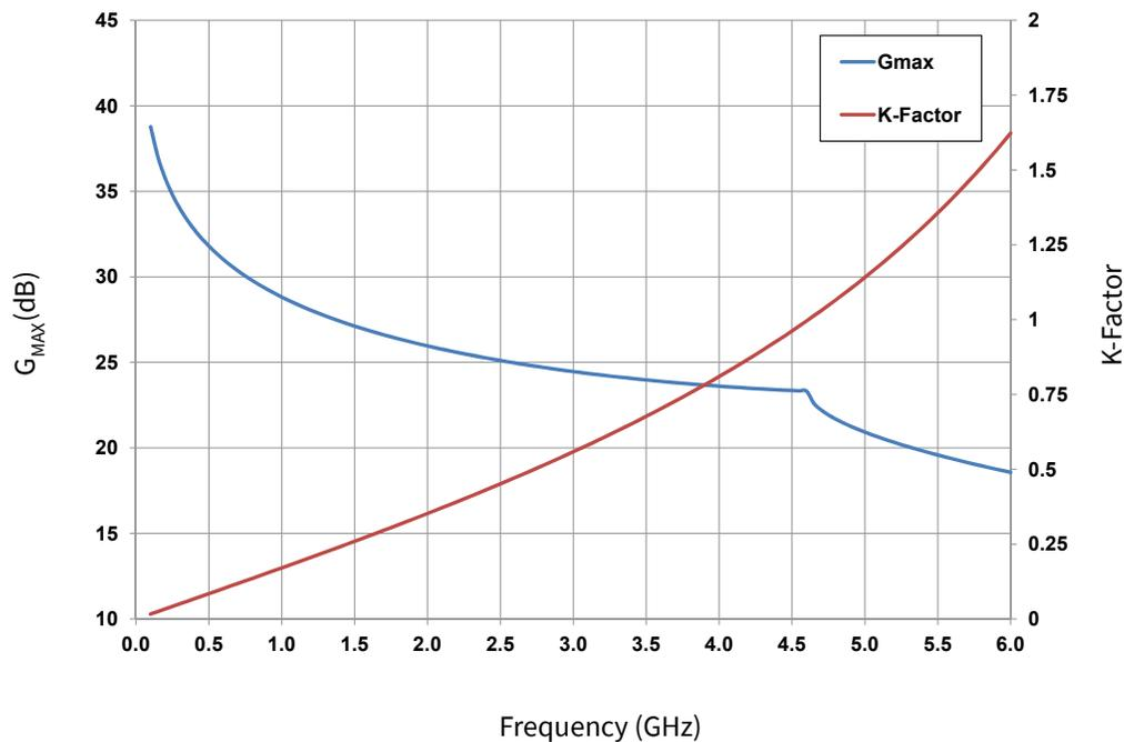
**Figure 16.**  $G_{MAX}$  and K-Factor vs Frequency
