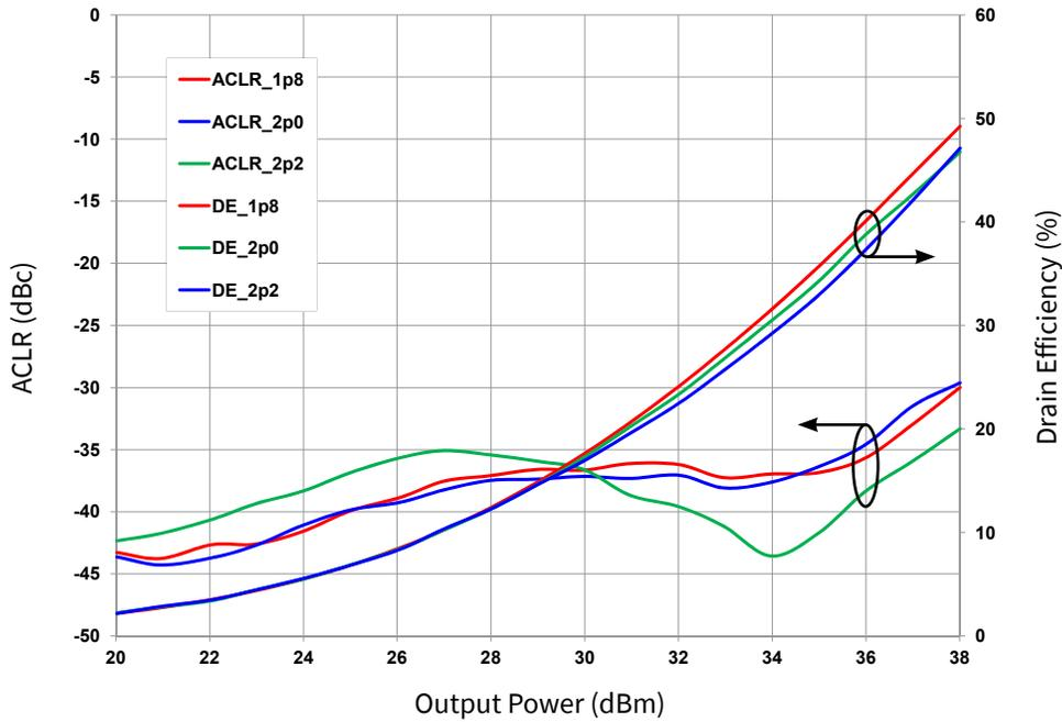
**Figure 8.** Typical Drain Efficiency and ACLR vs. Output Power
