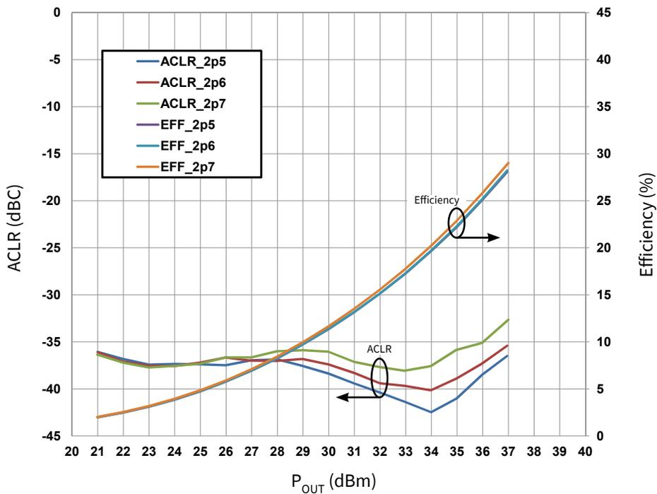
**Figure 2.** Typical Drain Efficiency and ACLR vs. Output Power
