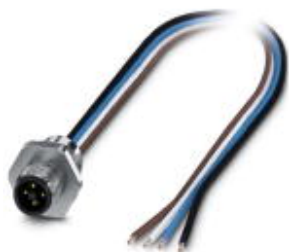
Flush-type connector, Power, 4-position, Plug, M12, T power, Front mounting, M16 x 1.5, Individual wires, cable length: 0.5 m
