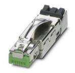
RJ45 connector, degree of protection: IP20, number of positions: 8, 10 Gbps, material: Zinc die-cast, connection method: IDC, connection cross section: AWG 23- 22, cable outlet: straight, High degree of resistance to vibration; 360° shielding; one-piece design; special tool-free assembly
