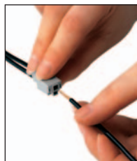
Solid conductor strip (8–9 mm) and connect conductor
