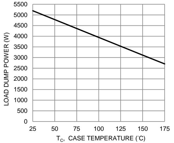
Fig. 2 Load Dump Power Characteristics (10ms Exponential Waveform)
