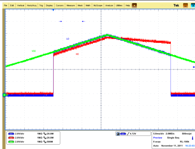
Figure 20. Negative 10-V Input
