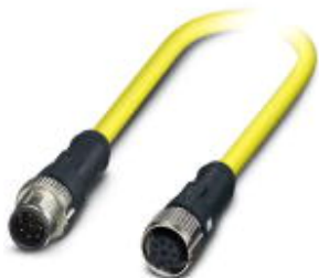
Sensor/actuator cable, 8-position, PVC, yellow, Plug straight M12 SPEEDCON, A-coded, on Socket straight M12 SPEEDCON, A-coded, cable length: 0.5 m
