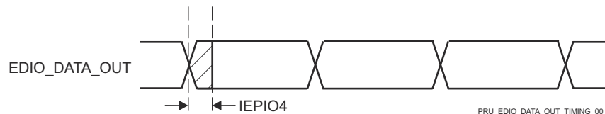
Figure 7-101. PRU_ICSSG IEP Digital IOs Timing Requirements
