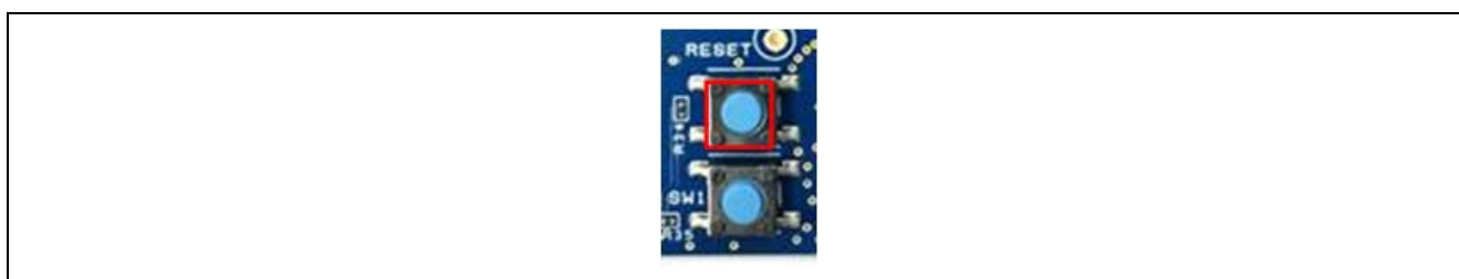
Figure 16. Reset Switch on EK-RA4W1 Board
