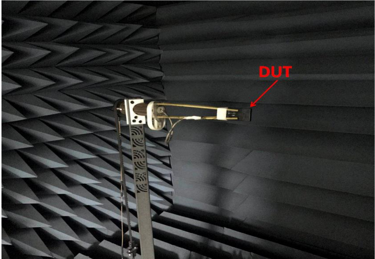
FIGURE4.1.3 ANTENNA LOADED WITH PC/ABS BLOCK OF 1MM THICKNESS TESTED IN OTA CHAMBER
