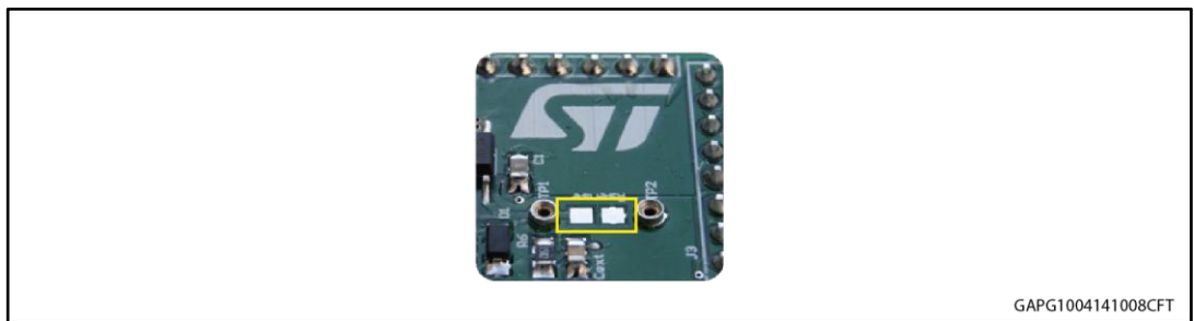
Figure 5: Pads for soldering SMD resistor
