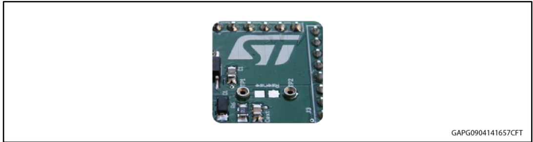
Figure 4: Mounting through-hole sense resistor
