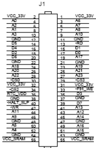
Figure 3. eZ80Acclaim! MDS Adapter Board Peripheral Bus Mini-Module Connector J1 Pin Configuration
